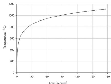
Figure 8: Standard time/temperature curve ISO 834
