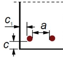
Fig. 1: Values for straight bars in beams and slabs (EN 1992-1-1) Note:  $c_d = \min(a/2, c_1, c)$
