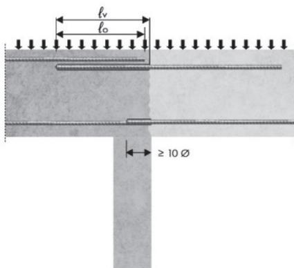
Figure 1: Overlap joint in slabs and beams
