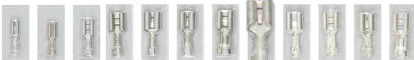
.... 995 5 0.5-1.0 mm 2 Plug: 2.8x0.5 mm with detent Tin-plated .... 992 3 0.5-1.0 mm 2 Plug: 2.8x0.8 mm Tin-plated .... 992 1 1.5-2.5 mm 2 Plug: 4.8x0.5 mm Tin-plated .... 991 9 0.5-1.0 mm 2 Plug: 6.3x0.8 mm Tin-plated .... 991 6 0.5-1.0 mm 2 Plug: 6.3x0.8 mm with detent Tin-plated .... 991 7 1.5-2.5 mm 2 Plug: 6.3x0.8 mm with detent Tin-plated .... 996 2 4.0-6.0 mm 2 Plug: 6.3x0.8 mm with detent Tin-plated .... 526 7 4.0-6.0 mm 2 Plug: 9.5x1.2 mm with detent Tin-plated .... 992 45 0.5-1.0 mm 2 Plug: 6.3x0.8 mm with detent Silver-plated .... 992 5 1.5-2.5 mm 2 Plug: 6.3x0.8 mm Silver-plated .... 992 8 1.5-2.5 mm 2 Plug: 6.3x0.8 mm with detent Silver-plated .... 992 6 4.0-6.0 mm 2 Plug: 6.3x0.8 mm Silver-plated
