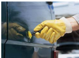
5. Using a hot air gun heat the adapter up to approx. 150°C and push it away to the side using the installation attachment.
