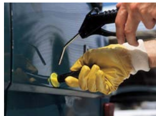
3. Glue adapter to deepest spot and cool using compressed air.
