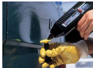
2. Install suitable adapter on installation attachment and apply special adhesive to centre.
