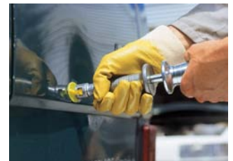
4. Hand sliding hammer into the adapter and straighten dent.
