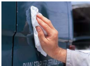
1. Clean dent using acetone cleaner.
